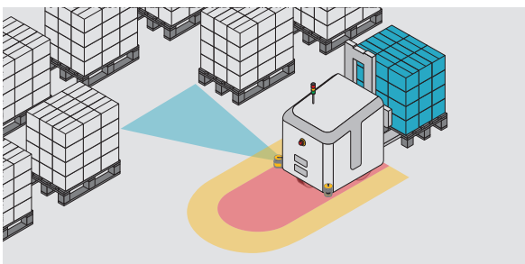
Direct navigation of AGVS thanks to monitoring of the environment.
